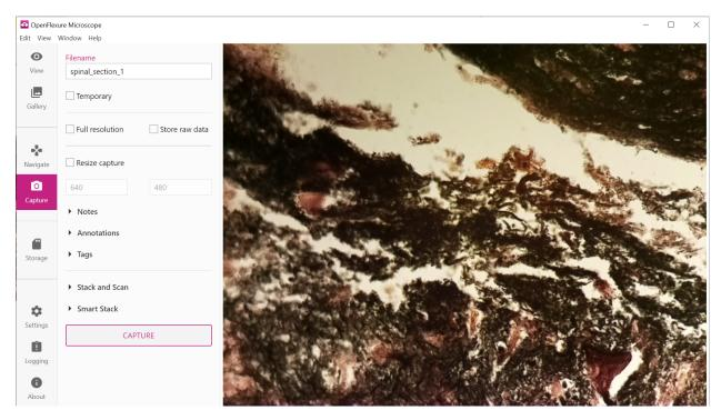
It is also possible to acquire a grid of images for stitching together into a mosaic, by expanding the "Stack and Scan" section and enabling the "Scan capture" checkbox. Scans are 3D by default (i.e. a mosaic of images in X and Y, with a Z stack at each position) but 2D or linear scans can be performed by setting the number of steps in the unused axes to 1. This allows XY mosaics or Z stacks to be performed.
