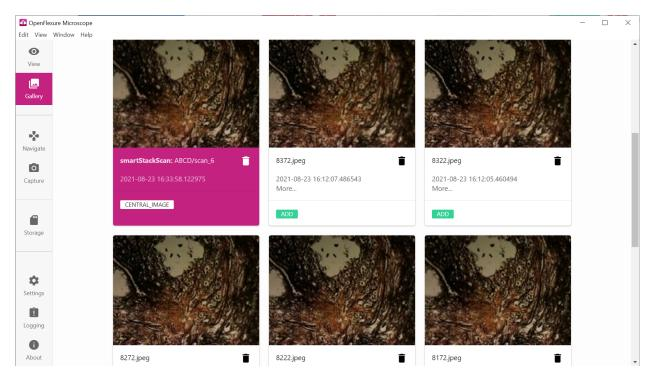
The gallery displays all the images currently stored on the microscope. Scans are grouped together into folders. Clicking on an image will display it in a "lightbox" view that allows scrolling through all images in the current view. When an image is displayed in the lightbox view, it may be right-clicked to download it. Multiple images can also be downloaded as a zip archive.
